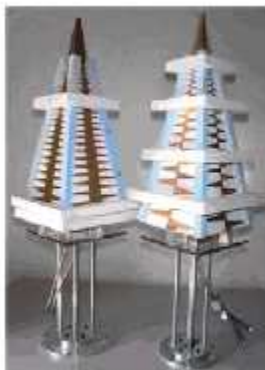
Figure A.3 — At left are wideband feeds developed for the ATA and at right is a wideband feed developed by TRW. Both have potential for 20:1 frequency range and have a maximum lateral dimension of approximately 1/2 at the wavelength of the lowest frequency of operation
